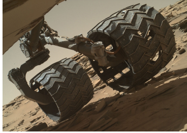
Figure 1: MSL image showing damage to the wheels from small rocks.
